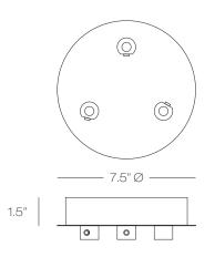
3 Light Strain Relief Round Canopy 7.5" Canopy with 3 strain relief ports. For 120V Fixtures, Braided Cloth or SVT Cord.
